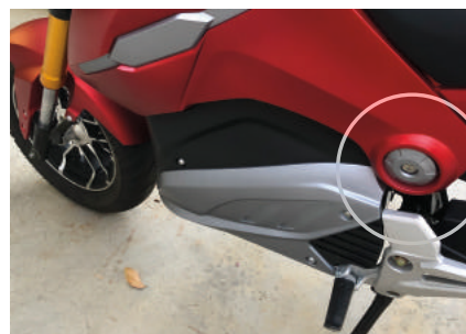
OPEN SEAT TO ACCESS BREAKER
