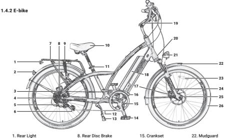
1. Rear Light 8. Rear Disc Brake 15. Crankset 2. Rear Reflector 9. Bungee Cord 16. Controller 23. Wheel Reflector 3. Motor 10. Saddle 17. Front Disc Brake 24. Front Fork 4. Freewheel 11. Saddle Quick Release 25. Quick Release 18. Battery 12. Chain 5. Rear Derailleur Protector 19. Adjustable Stem 26. Tire 6. Rear Derailleur 13. Kickstand 20. Frame Number
